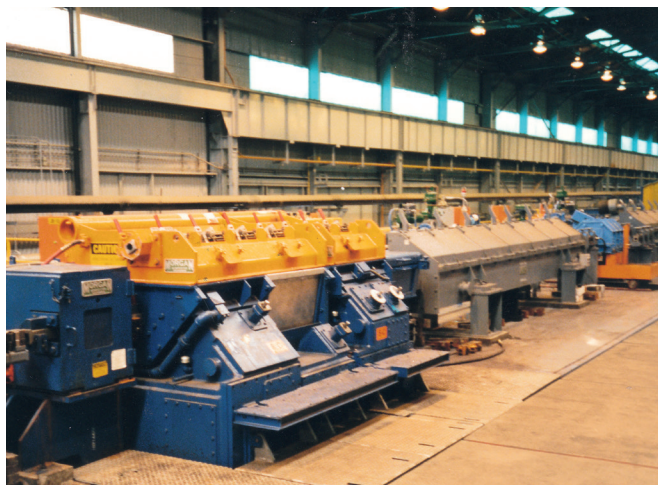
A Morgan Reducing/Sizing Mill from Primetals Technologies in a wire rod mill
